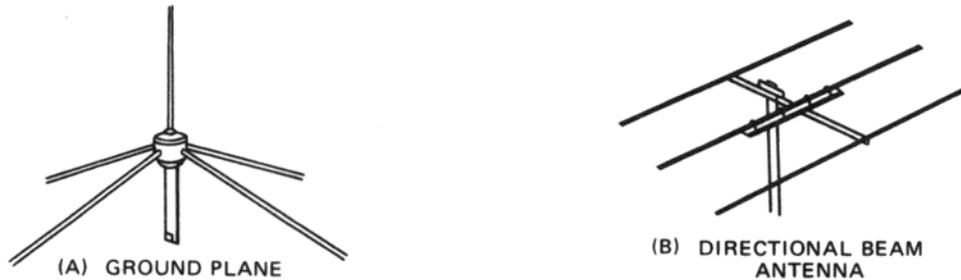
FIGURE 8. BASE STATION ANTENNAS
