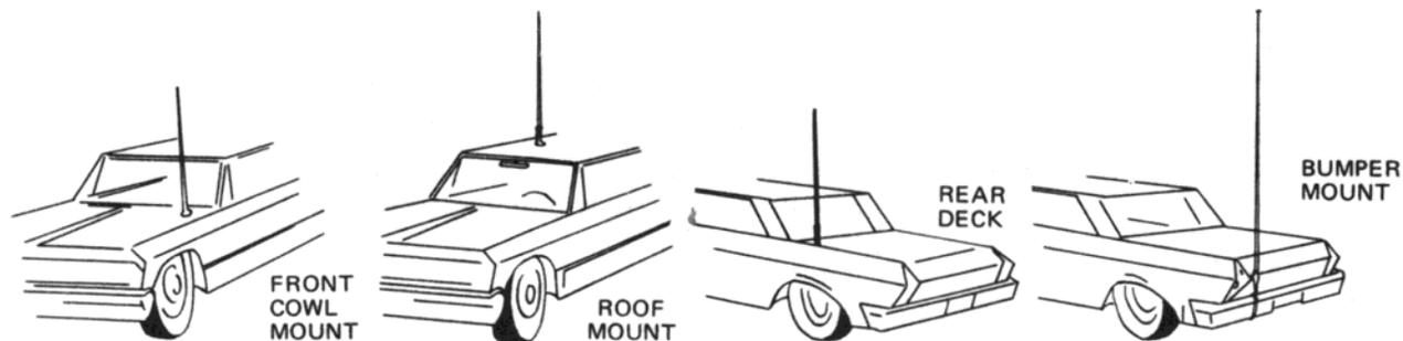
**FIGURE 7. MOBILE ANTENNA MOUNTING**
