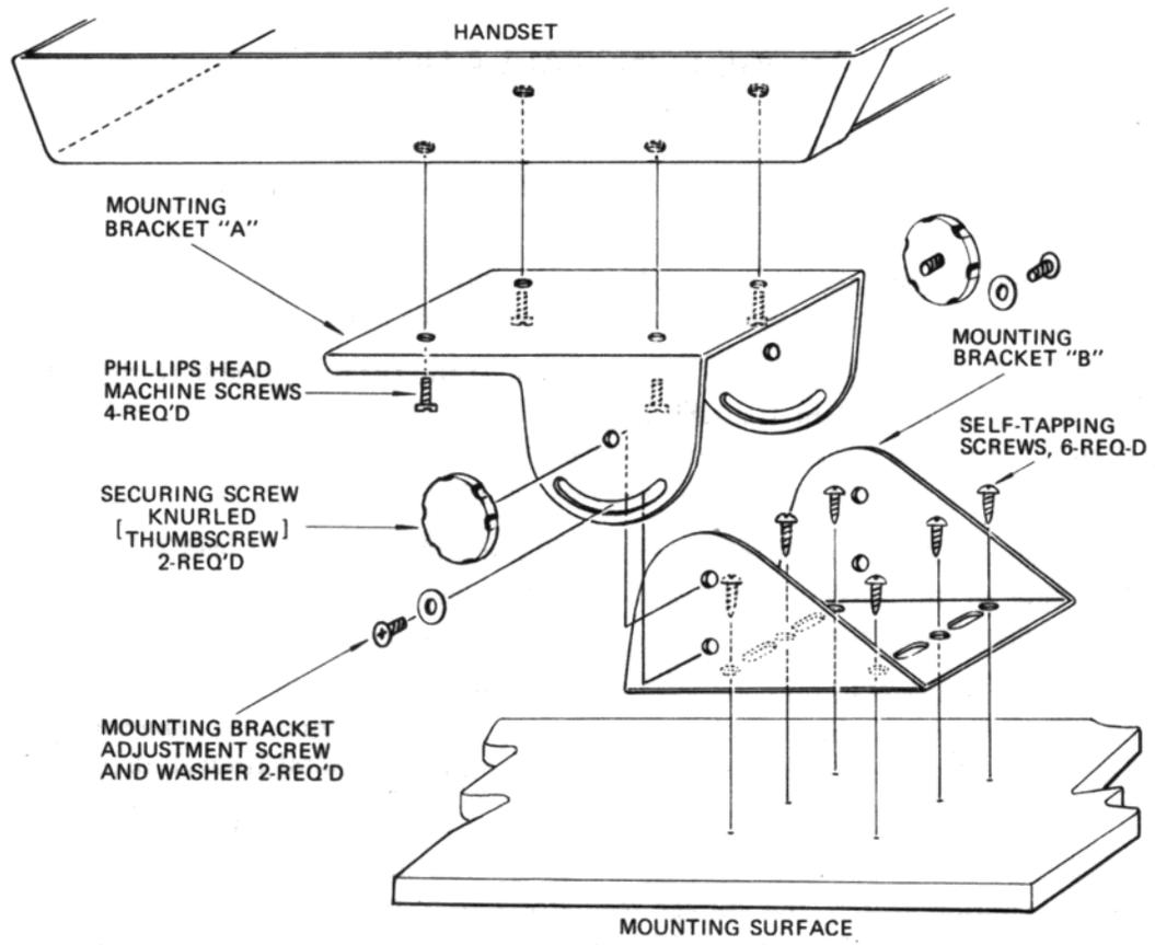
**FIGURE 1. TRANSCEIVER MOUNTING, EXPLODED VIEW**
