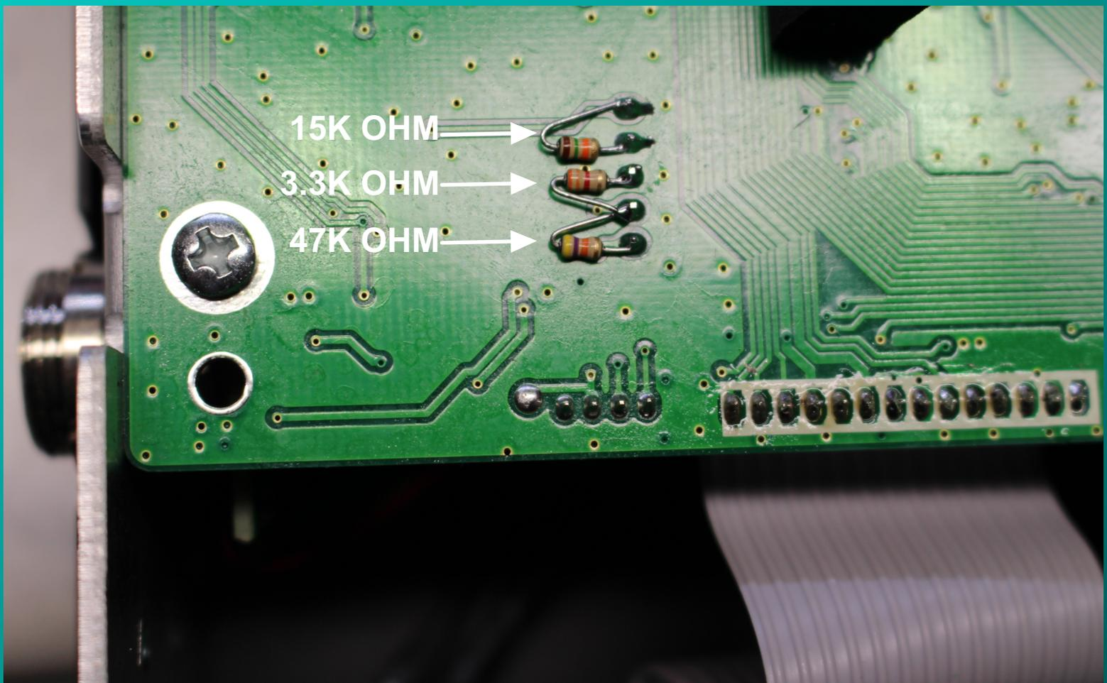
The echo ON/OFF portion of the control still works, the only difference is the effect stays the same and will never go out of adjustment.
