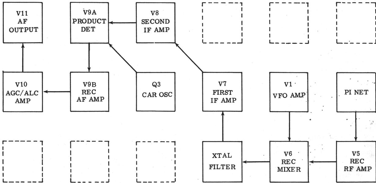
FIGURE 2. BLOCK DIAGRAM, RECEIVE MODE
