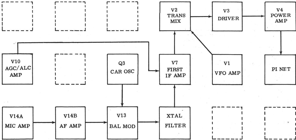
FIGURE 1. BLOCK DIAGRAM, TRANSMIT MODE
