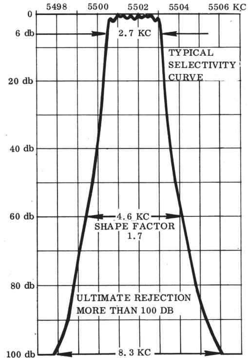
FIGURE 3. CRYSTAL FILTER CHARACTERISTICS
