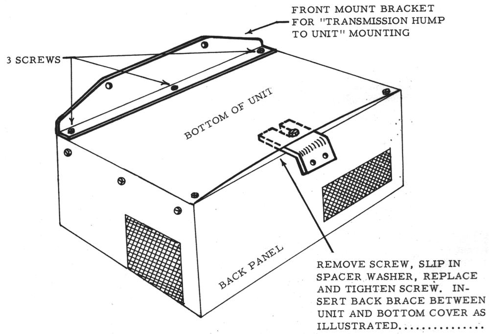
FIGURE 4. MOBILE INSTALLATION MOUNTING DETAILS
