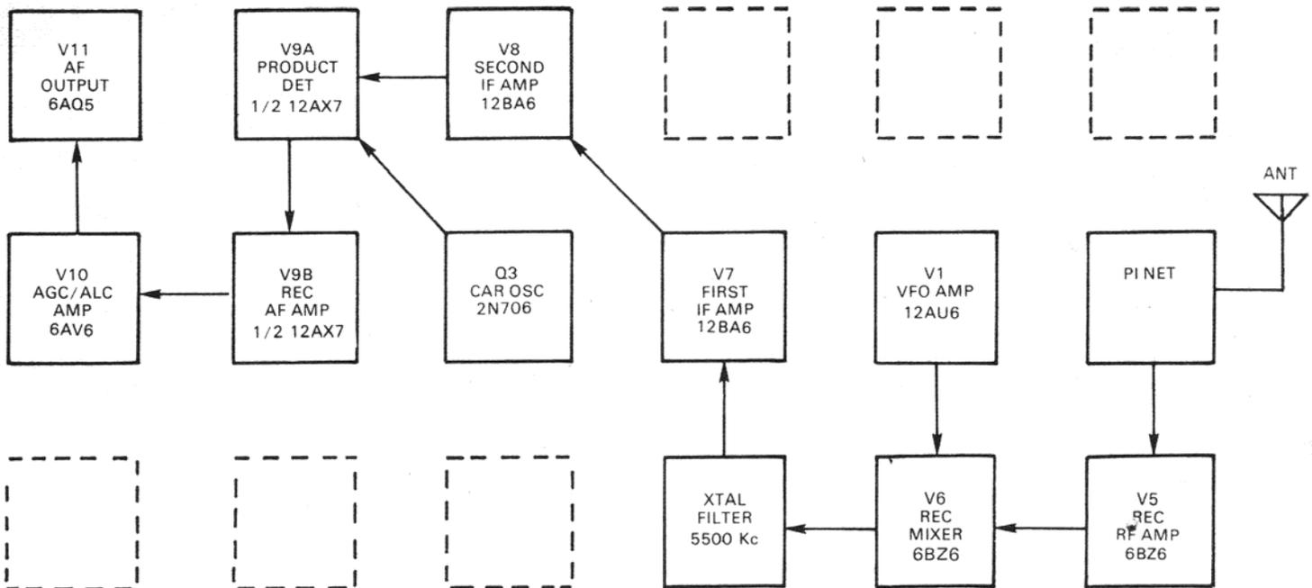
**FIGURE 5. BLOCK DIAGRAM, RECEIVE MODE**
