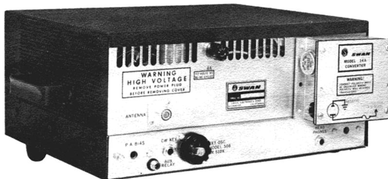
FIG. 2. SWAN CYGNET MODEL 1011, REAR VIEW, WITH 14-A D.C. CONVERTER ATTACHED.
