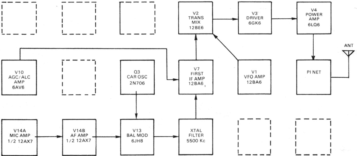
**FIGURE 4. BLOCK DIAGRAM, TRANSMIT MODE**
