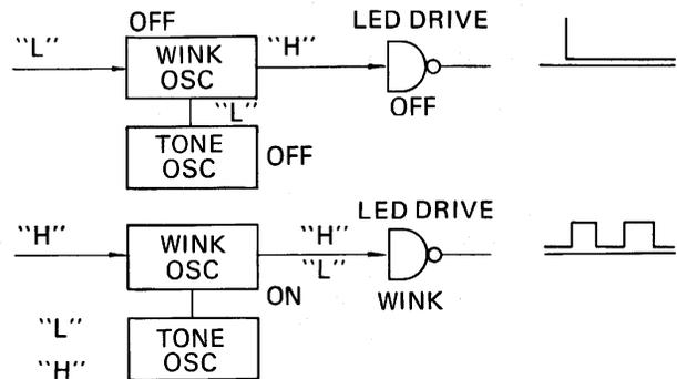
Figure 3. Operation of Wink Osc When Its Input Is "Low" and "High".
