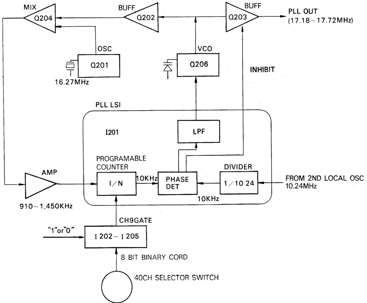
Figure 1. Block Diagram for PLL Synthesizer Circuit.
