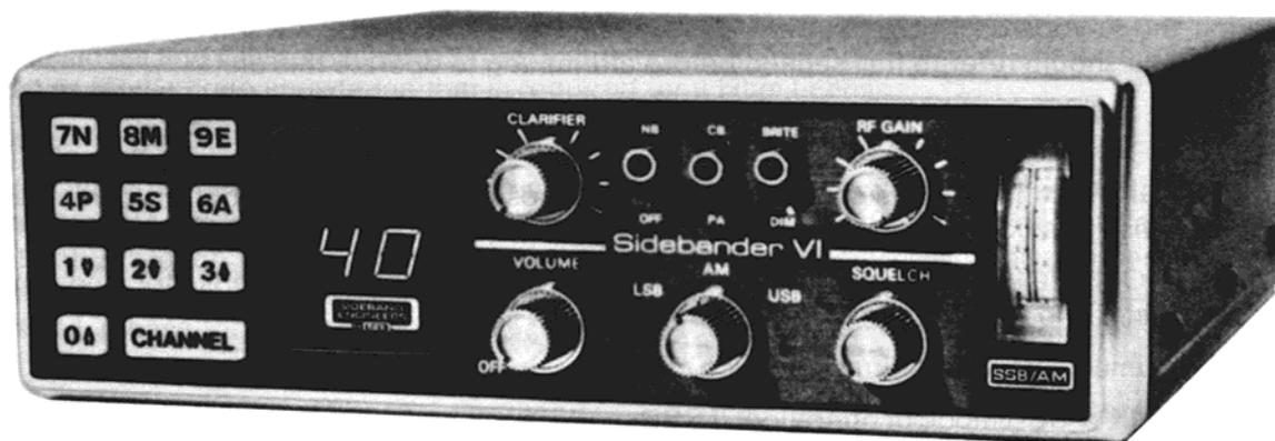
1. OFF/ON VOLUME CONTROL — turns the radio on and adjusts the volume received audio.
