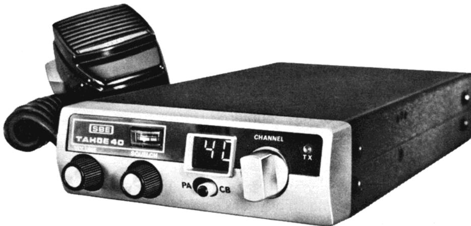
4. TX Light - Indicates when the transmitter is on (keyed).
