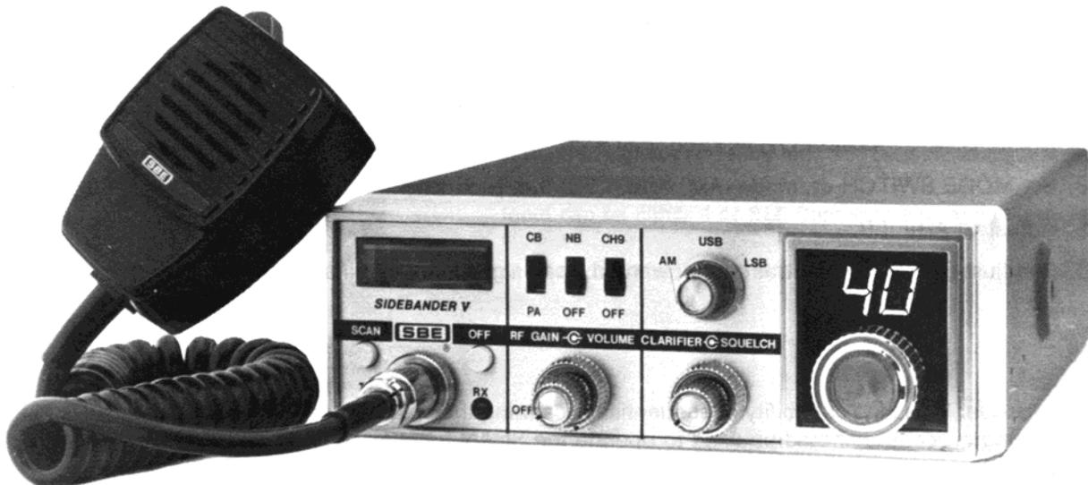
3. **SQUELCH** — The Squelch control blanks out unwanted noise when no signals are present. Turn this control fully counterclockwise then slowly clockwise until the receiver noise disappears. Any signal to be received must now be slightly stronger than the average received noise. Further clockwise rotation will increase the threshold level which a signal must overcome in order to be heard. Only strong signals will be heard at the maximum clockwise setting.
