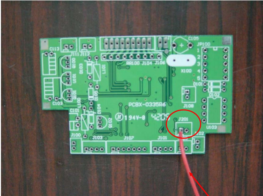
The red wire (which is originally connected to first lead of IC-358 of the module board mounted on PCBX-0335R3) is to be connected to the left hole of J-201 on the PCBX-0335R6.
