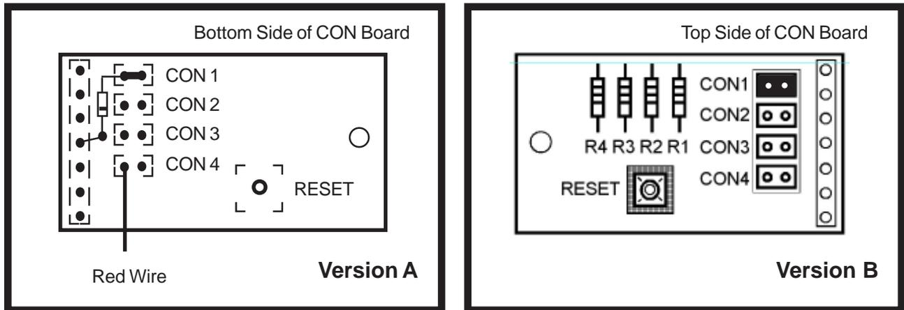
The CON Board is located on the right front side of the radio (Behind the Mic Jack)
