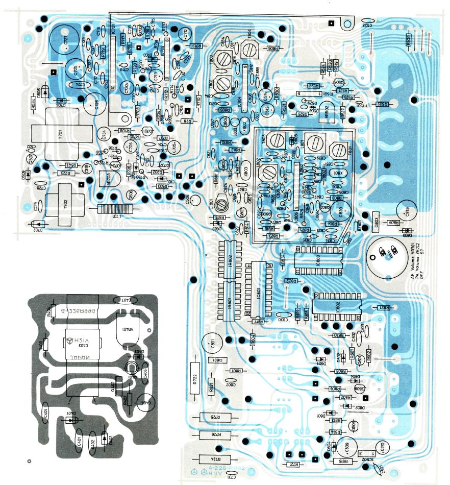
NOTE: MARKS INDICATE PLATED-THROUGH HOLES/PINS. THUS, SURFACE-A AND SURFACE-B ARE CONNECTED AT THOSE POINTS.
