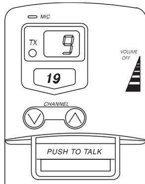
1. Turn **VOLUME** clockwise until it clicks to turn on the CB. The CB automatically tunes to Channel 9, the emergency channel.
