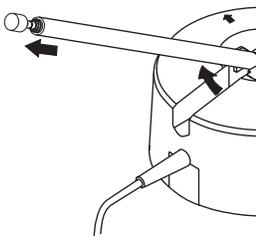
**Note:** Fully extend the antenna for maximum range.
