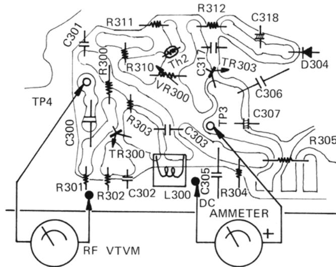
NOTE: 1. Connect DC Ammeter and RF VTVM to TP3 and TP4 on the Main P. C. Board.
