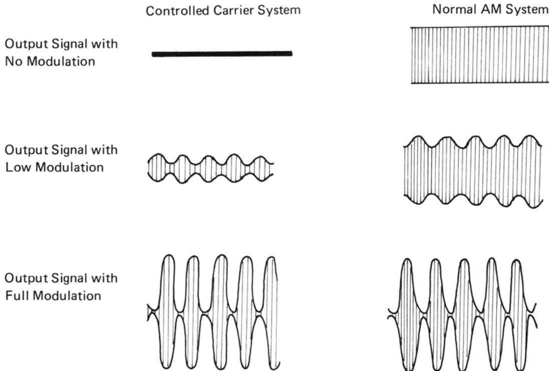
By controlling the carrier power which is transmitted in accordance with the level of the modulation input signals, it is possible to reduce the amount of power used when transmitting (and thus prolong the life of the batteries).
