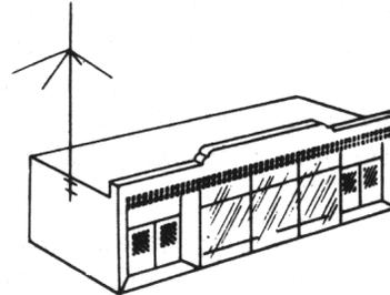
to connect the antenna to the RADIO-PHONE. For cable runs longer than 75 feet, RG-8/U cable is preferred to minimize the power loss. Each end of the cable must be terminated in a UHF connector, PL-259. If RG-58/U cable is used, a type UG-175/U adapter is also required. See Figure 1 for connector assembly instructions.
