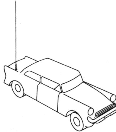
The 555579 antenna, supplied with a swivel ball mounting, is designed to be mounted through any surface of the vehicle. A twenty foot lead-in cable and gutter clip is also supplied with this antenna.
