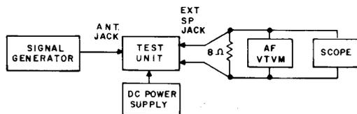
Figure 9 – Test Equipment Hook-Up – Receiver
