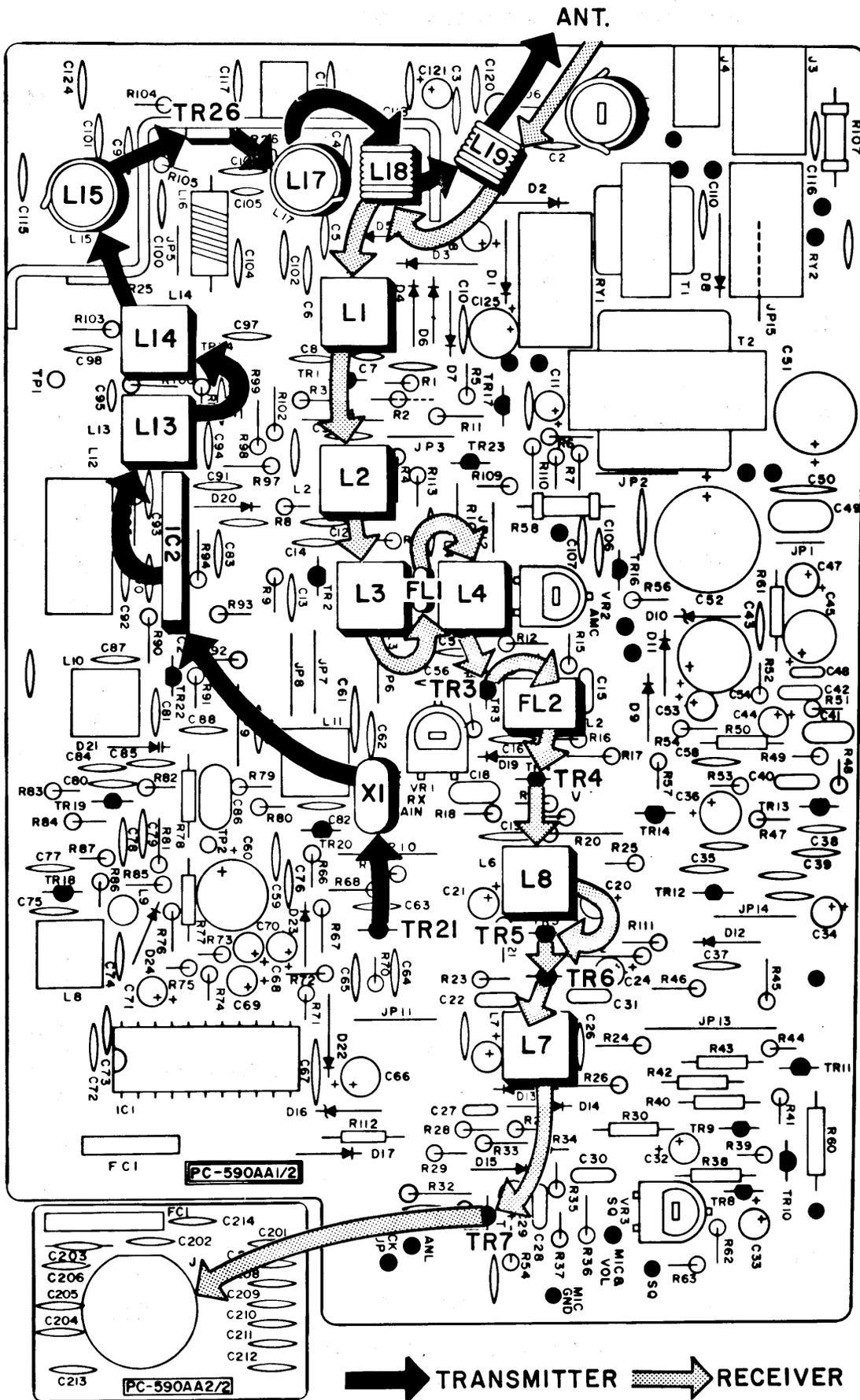
Figure 6 - Transceiver Signal Paths
