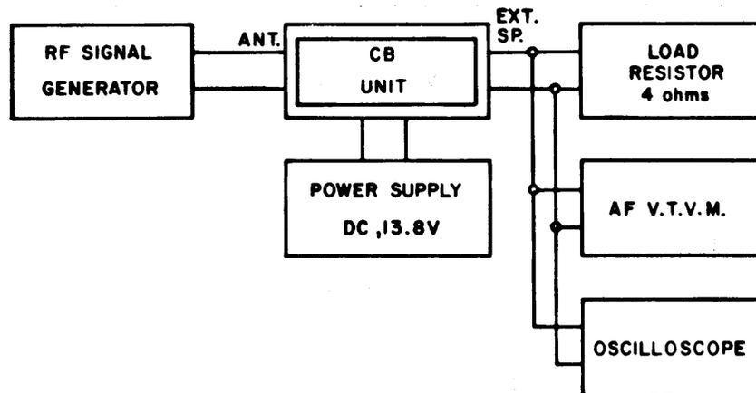
Figure 2 – Receiver Alignment Test Equipment Set-Up
