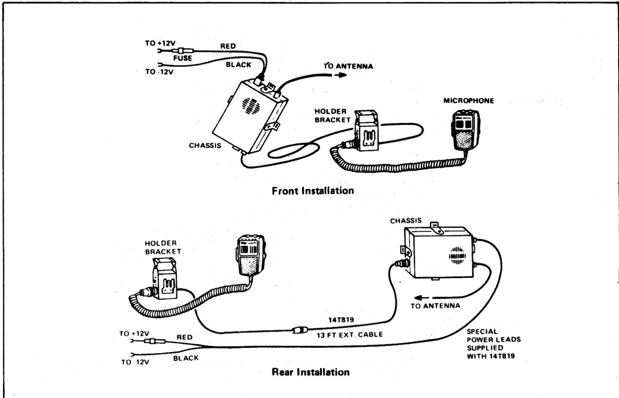
Figure 9. 14T275 Cable Interconnections
