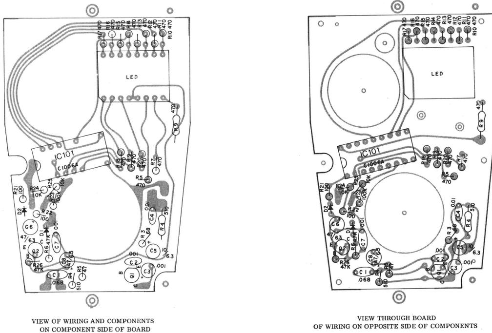
Figure 4. Mic/Spaker/Control Board (Foil on Both Sides)
