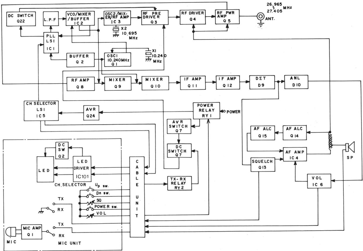
Figure 3. Overall Block Diagram, 14T275 CB Transceiver
