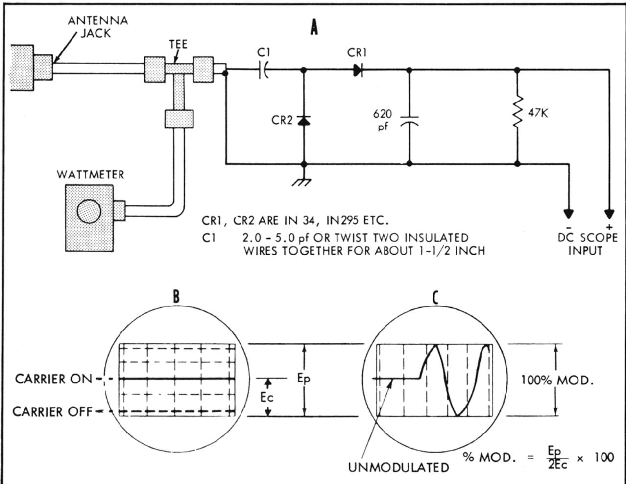
Figure 3-3 Modulation Detector
