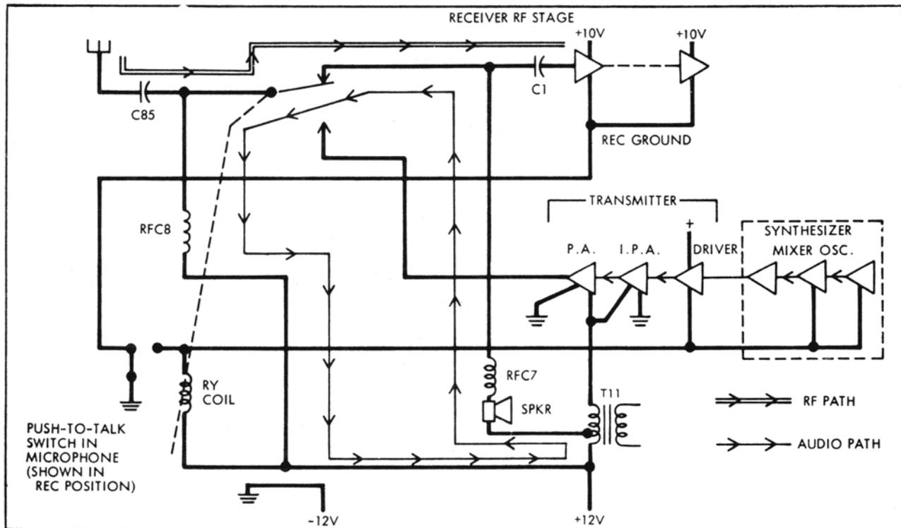
Figure 2-2 Transmit-Receive Switching Schematic
