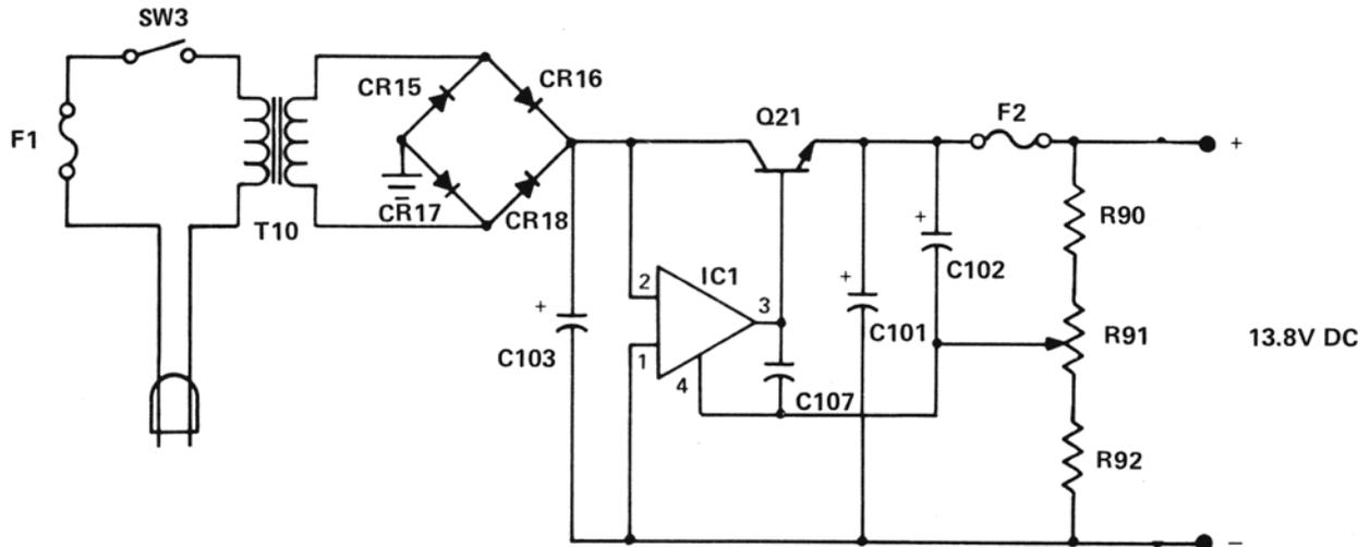
Figure 2-3 Power Supply Circuit
