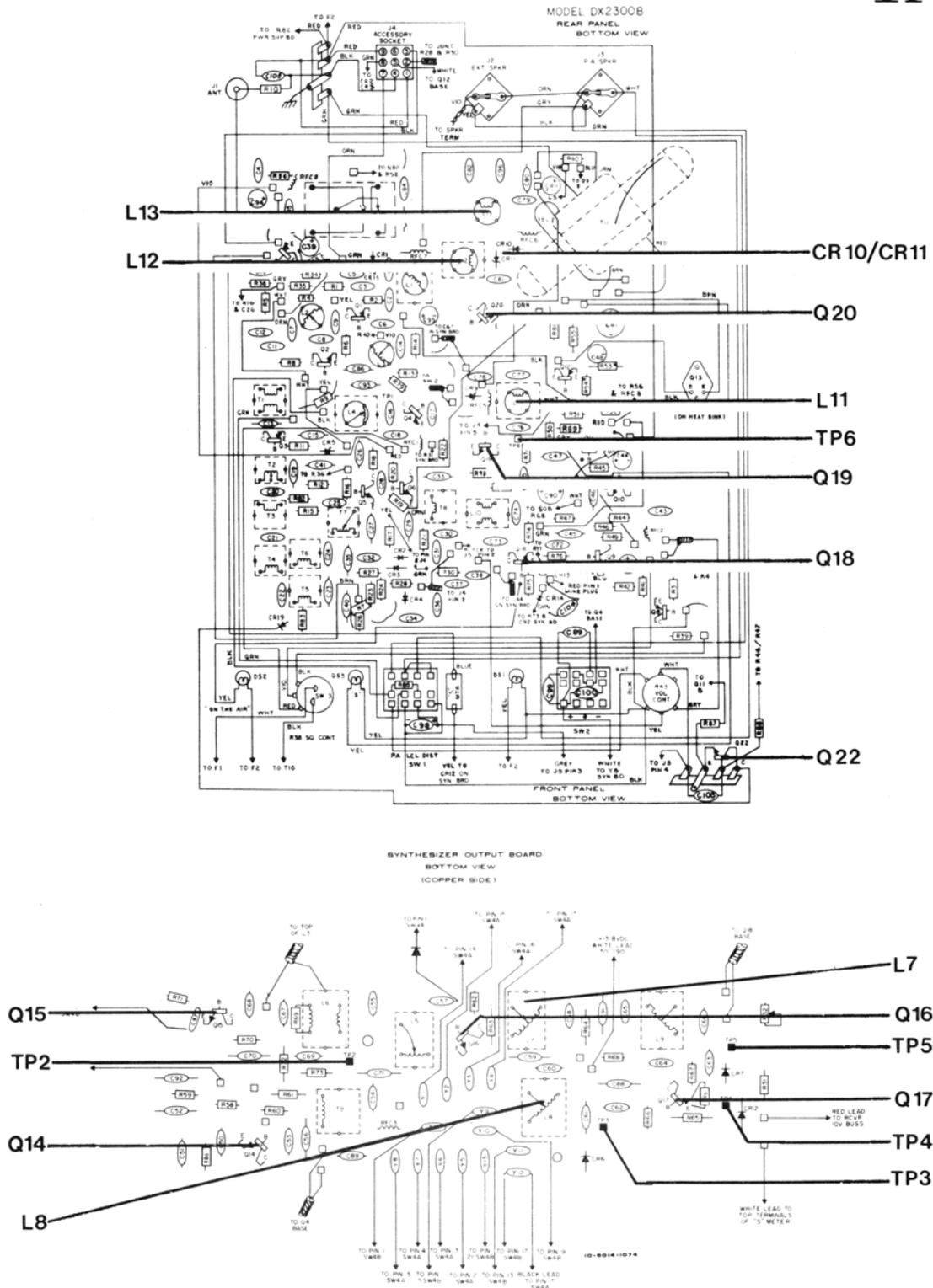
Figure 3-5 Test Point Locations for Transmitter Troubleshooting
