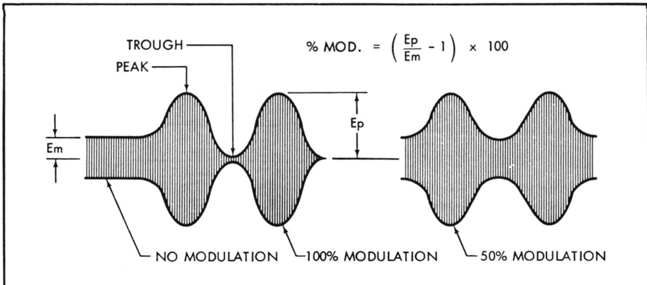
Figure 3-4 Direct Modulation Monitor
