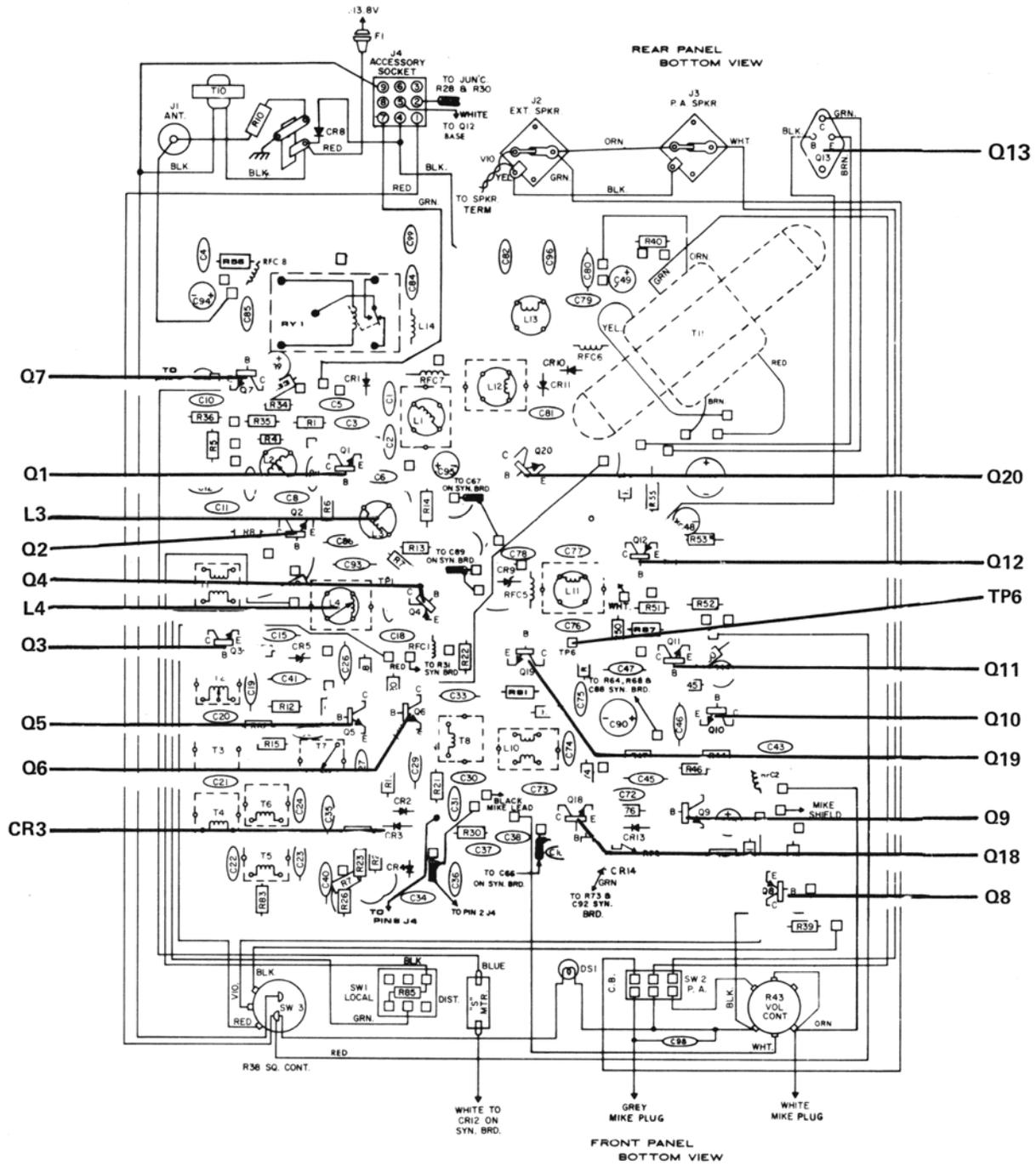
Figure 3-1 Test Point Locations for Voltage Charts
