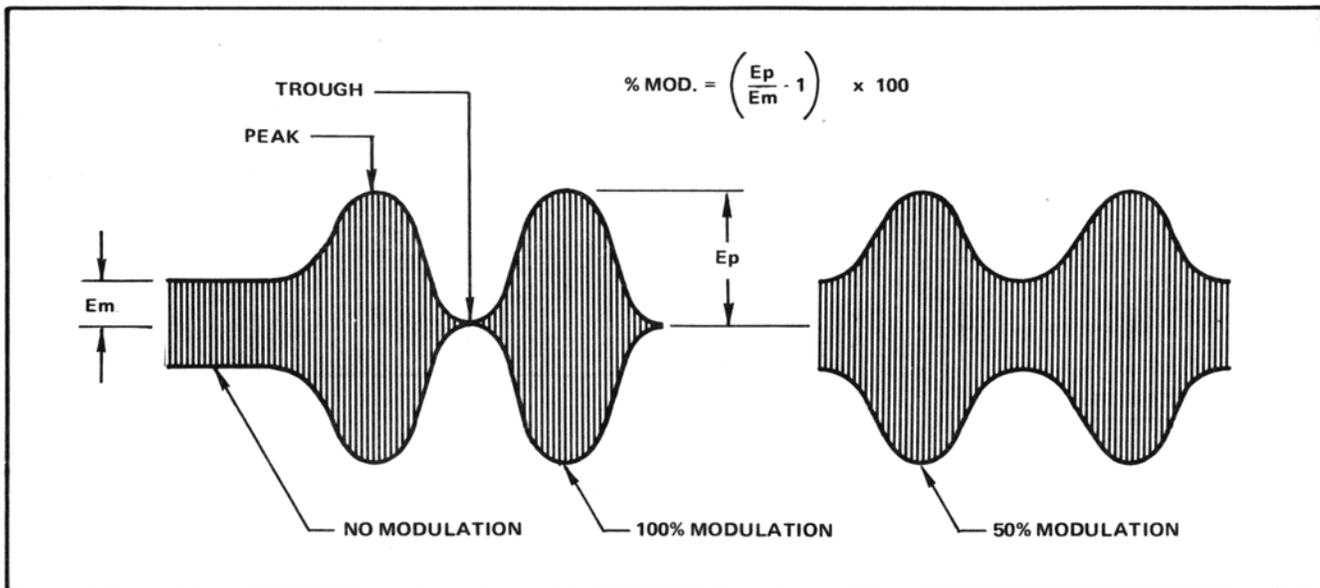
Figure 4-2 Direct Modulation Monitor
