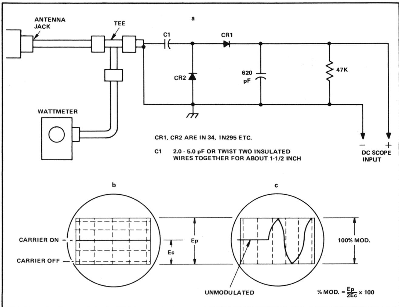
Figure 4-1 Modulation Detector
