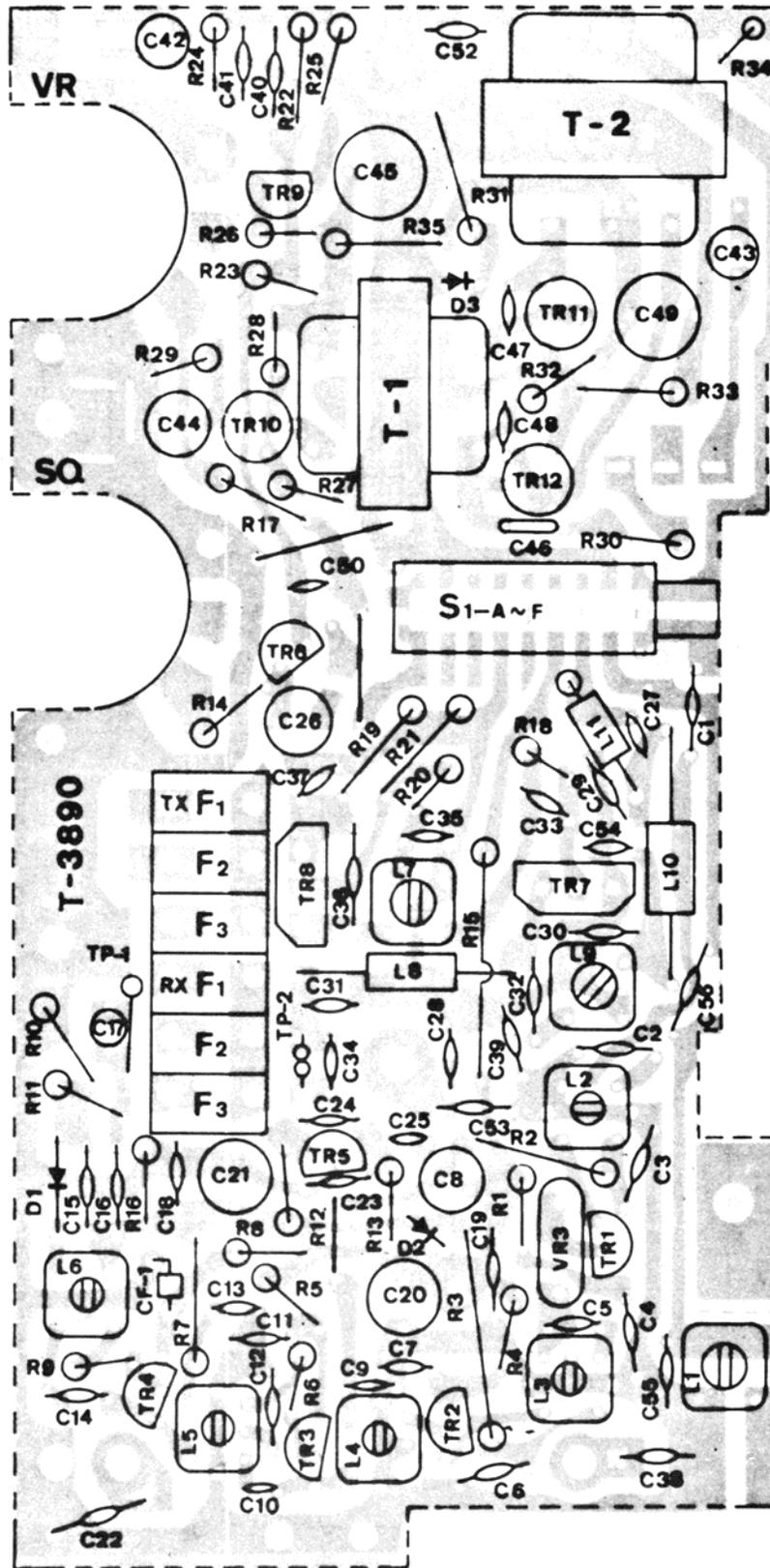
Figure 6-1 Parts Locator (All Models)
