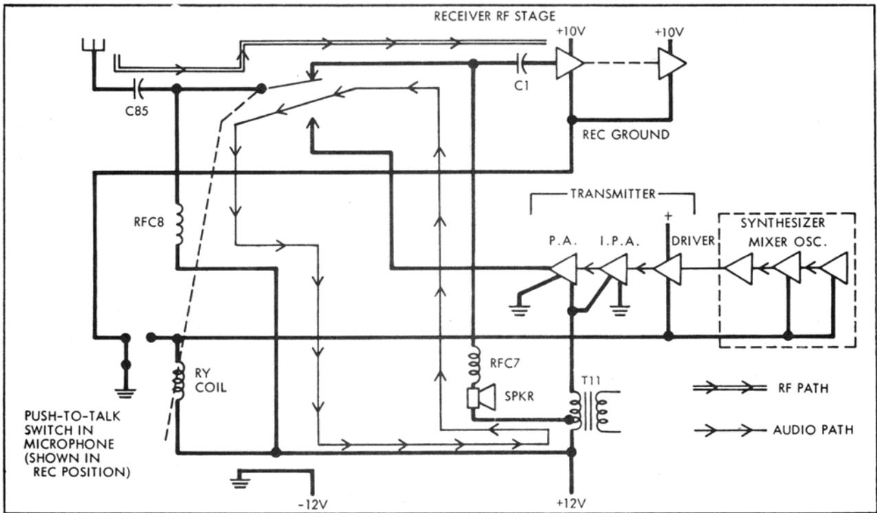
Fig. 1 RECEIVE-TRANSMIT SWITCHING SCHEMATIC
