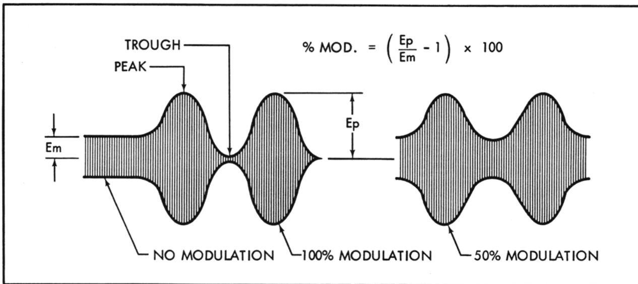
Figure 3-2. Direct Modulation Monitor
