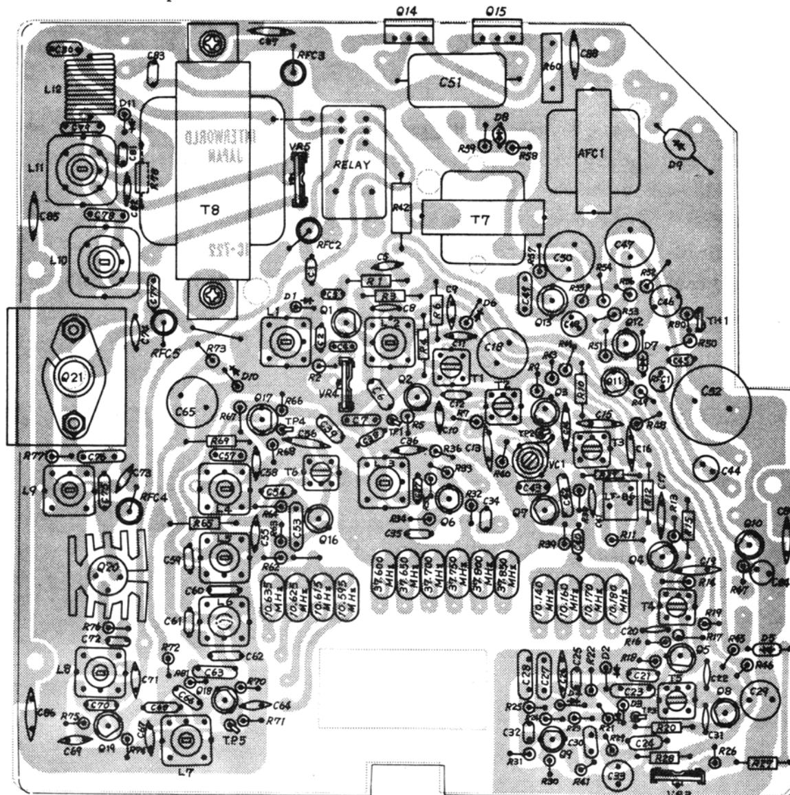
Figure 5-1. Parts Locator (Component Side)
