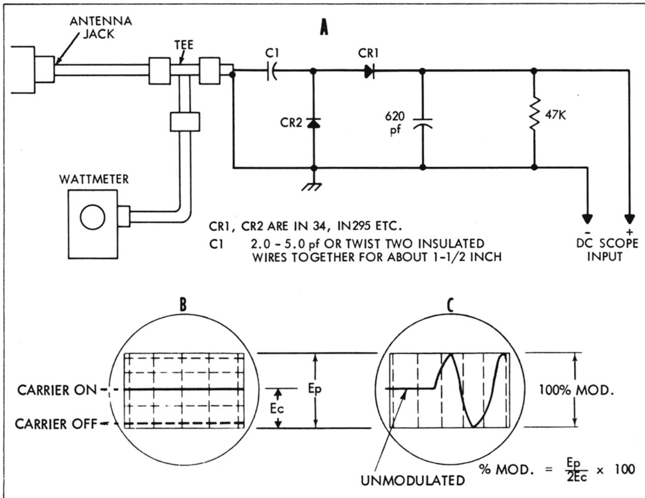
Figure 3-1. Modulation Detector
