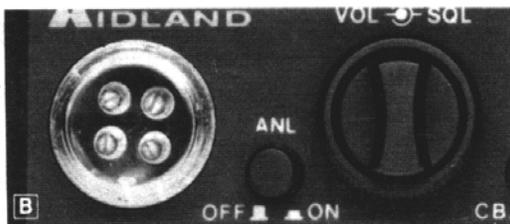
**B Microphone Connector.** Securely links your microphone to the main unit during use.
