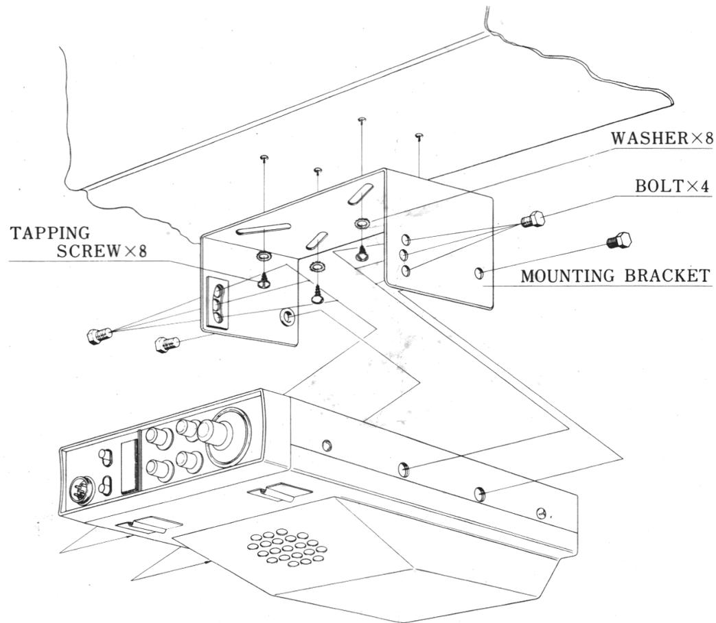
Safety and operating convenience are the primary factors to be considered when mounting any piece of equipment in an automobile. Be sure that the transceiver controls may be easily reached by the operator. Also be sure that connecting cables do not interfere the operation of the brake, accelerator, etc.
