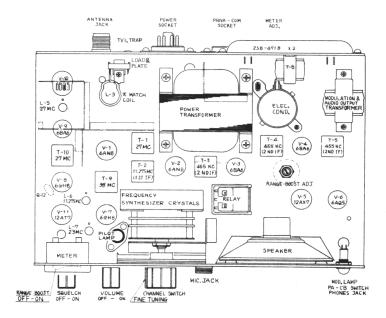
Adjust the top and bottom tuning cores of T3, T4 and T5 for maximum output. Reduce generator output progressively as circuits come into line so that VTVM reading does not exceed about 0.5 volts. When no further increase can be obtained by adjusting the cores, disconnect the signal generator and proceed with the 11.275 Mc IF adjustments.
