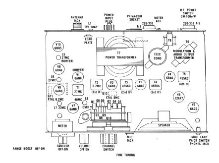
Adjust the top and bottom tuning cores of T3, T4 and T5 for maximum output. Reduce generator output progressively as circuits come into line so that VTVM reading does not exceed about 0.5 volts. When no further increase can be obtained by adjusting the cores, disconnect the signal generator and proceed with the 6.2 Mc IF adjustments.
