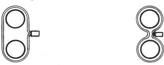
between the coils to tighten. Do not twist the ends of the loop with respect to each other-leave as a flat loop as shown.
