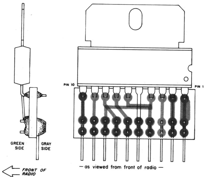
**Figure 4-4. Audio IC Mounted on Extender P.C. Board**
