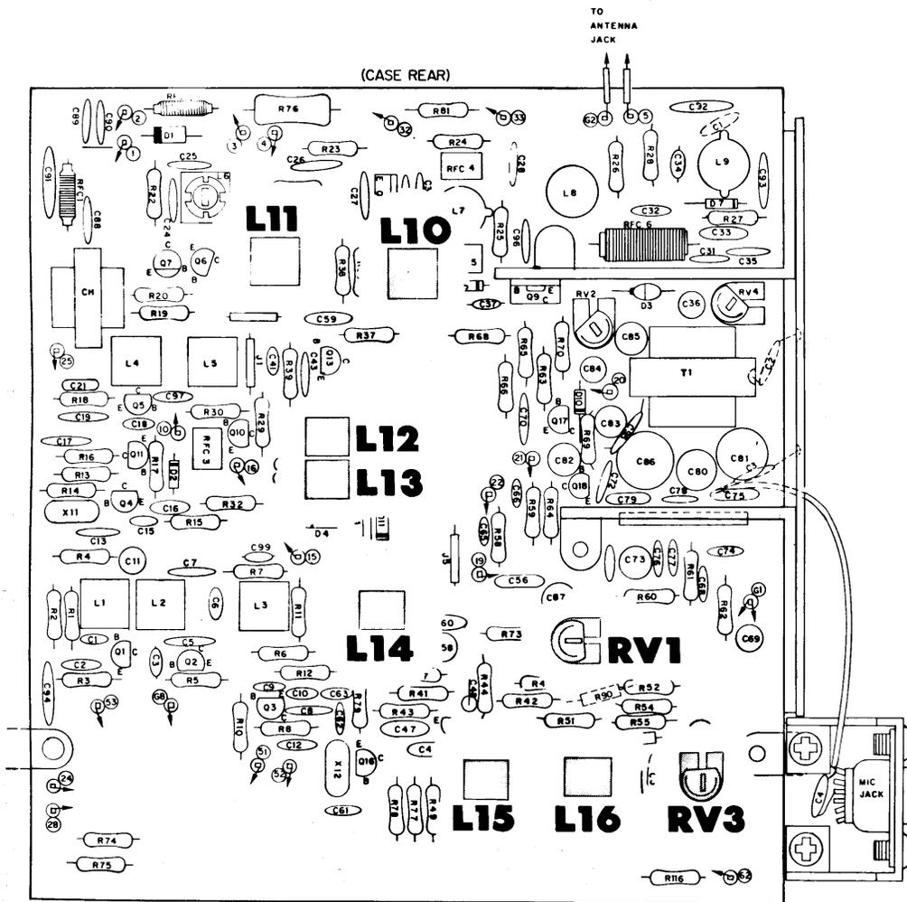
Figure 3-7. Components Adjusted for Receiver Alignment
