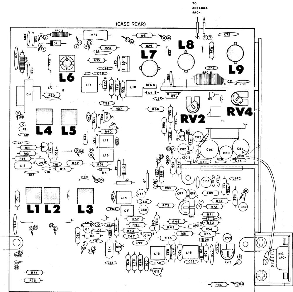
Figure 3-6. Components Adjusted for Transmitter Alignment
