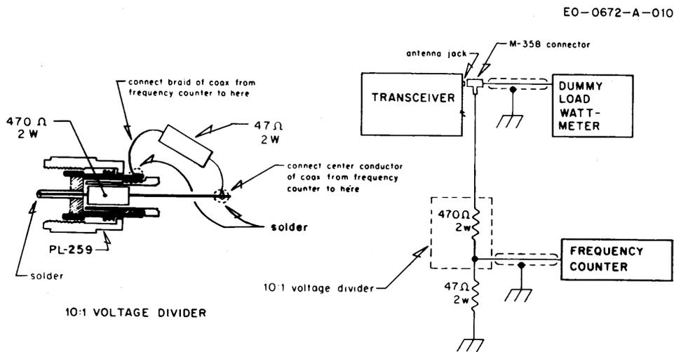
Figure 3-4. Connection of Frequency Counter and Dummy Load
