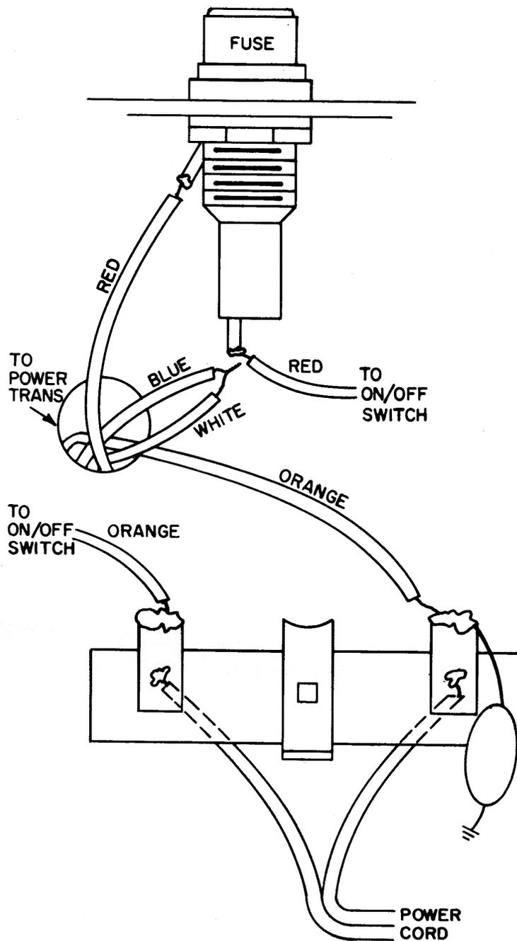
Figure 3-2. After Wiring Model 3084 for 240 VAC
