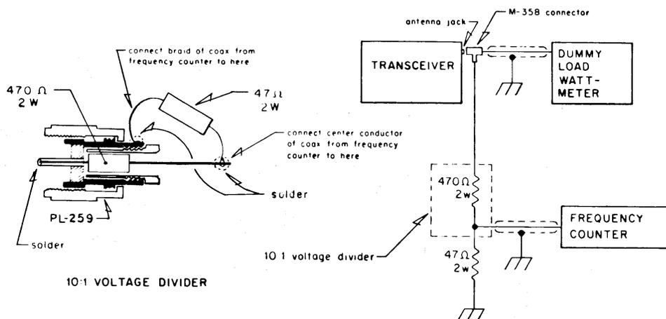
**Figure 3-3. Connection of Frequency Counter and Dummy Load**
