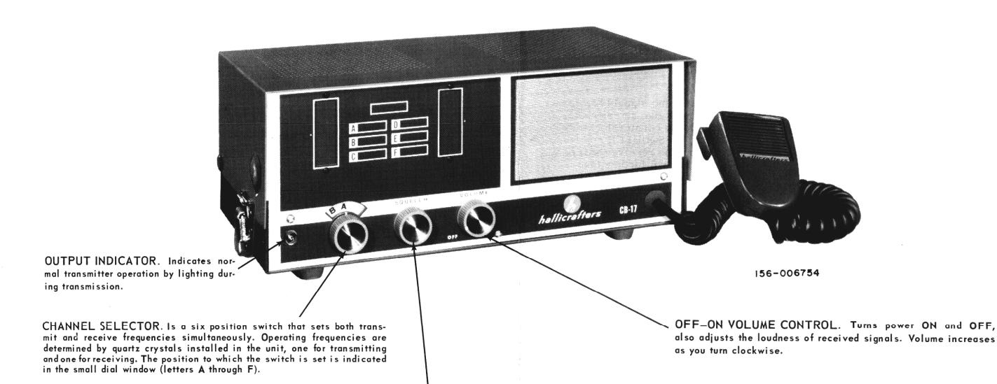
SQUELCH CONTROL. Quiets background noise (static) in the absence of a signal. In the fully clockwise position, the transceiver is unsquelched (i.e., no noise quieting). In the fully counterclockwise position, the unit is fully squelched. In practice, this control should be set to the point that just quiets the noise.
