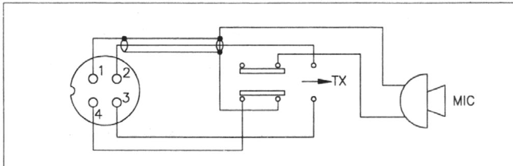
If the microphone to be used is provided with pre-cut leads, they must be revised as follows :
