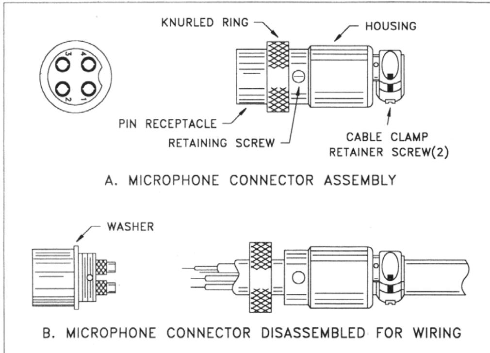
To wire the microphone cable to the plug provided, proceed as follows :
