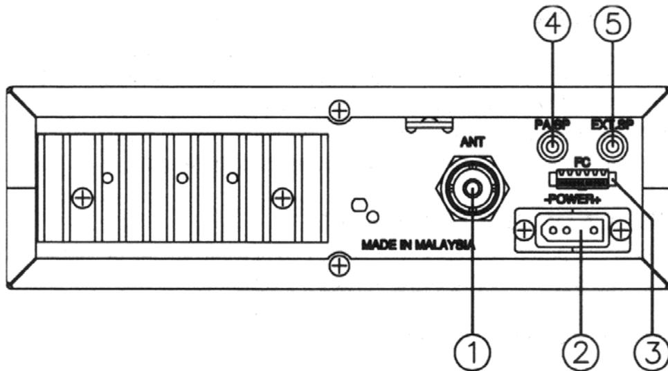
1. **ANTENNA** : This jack accepts 50 ohms coaxial cable with a PL-259 type plug.
