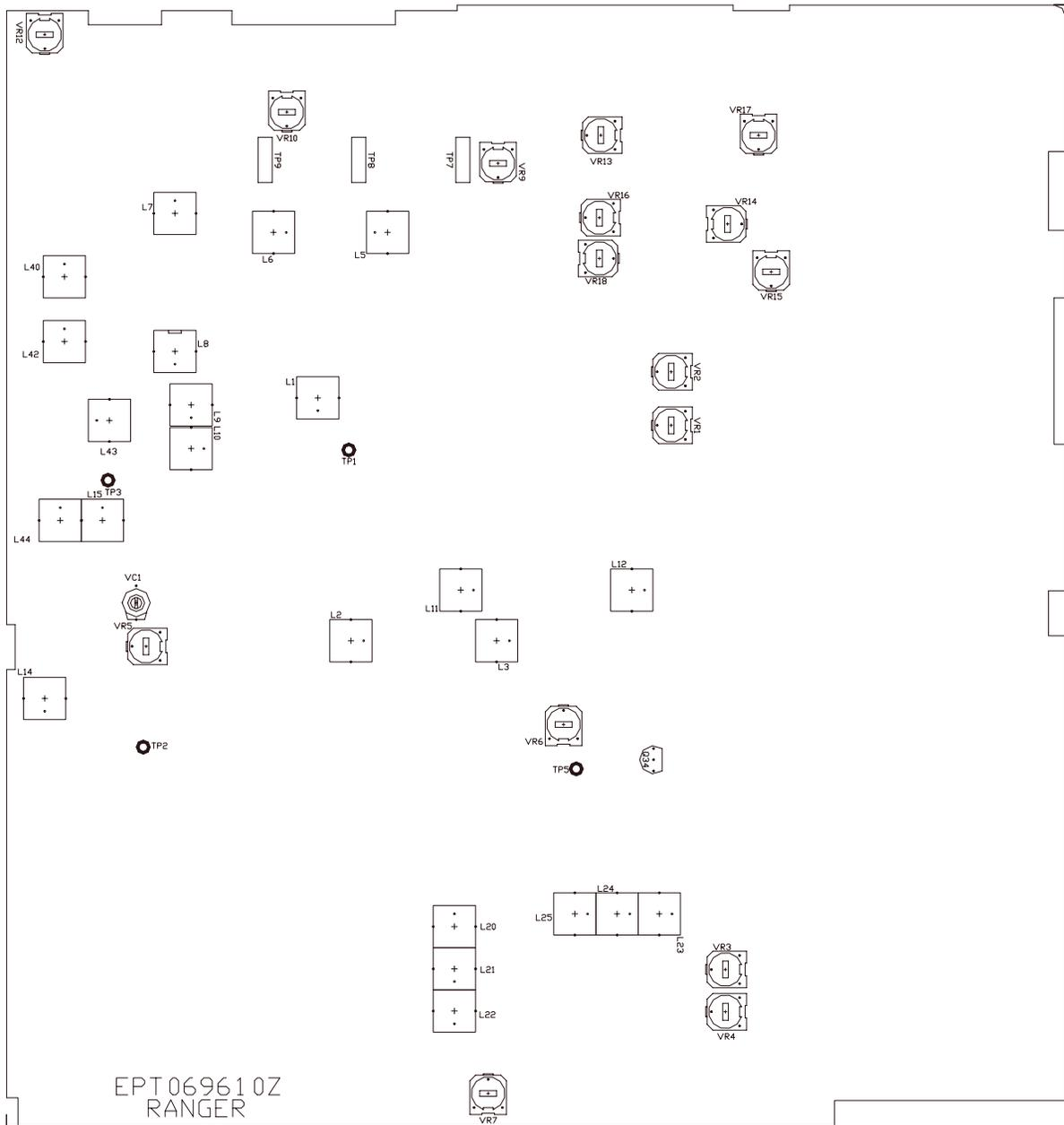
Figure 4-3 Main PCB Adjustment Location
