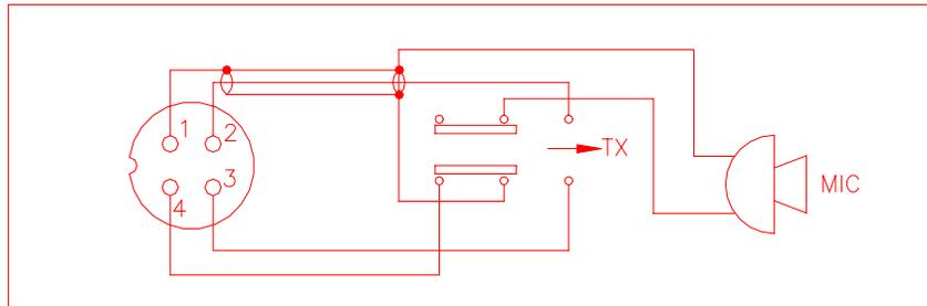
Figure 2-3 Your Transceiver Microphone Schematic
