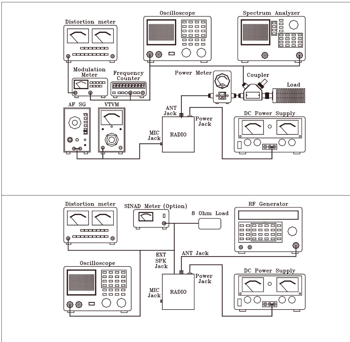
Figure 4-2 Receiver test setup
