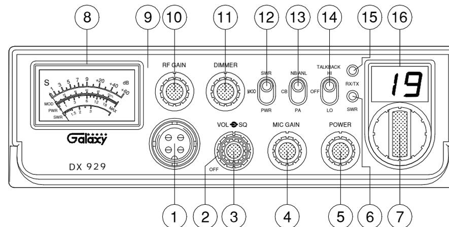
1. **MICROPHONE JACK:** Used to connect microphone for voice source.
