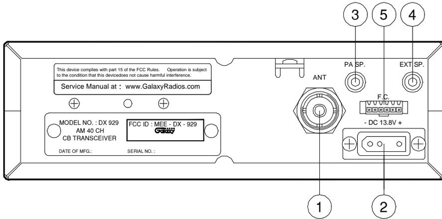
1. **ANTENNA:** This jack accepts a 50-ohm coaxial cable with a PL-259 type plug.
