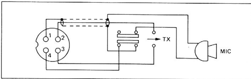
Fig. 3. 侍 samurai microphone schematic.
