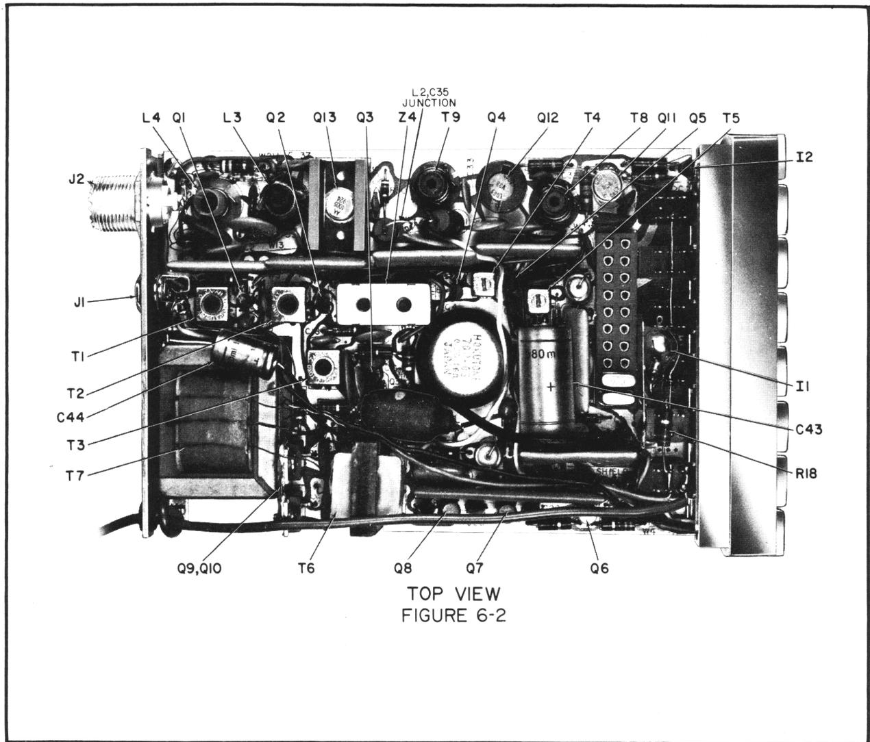
by starting with the slug at the top of the coil and tune through the peak RF reading to  $0.125 \pm 0.025$  volts RF on the emitter of Q2. Check for starting and uniform injection voltage on the channels used.
