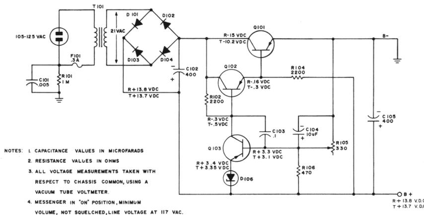
**AC POWER SUPPLY SCHEMATIC
