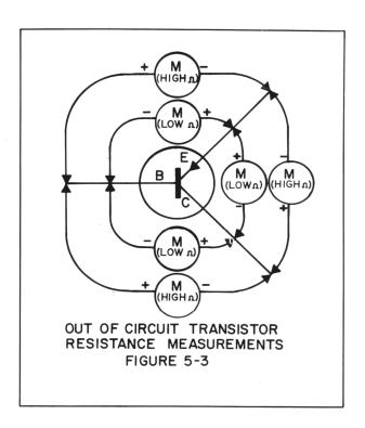
Polarities shown in Figure 5-3 are for PNP transistor types. For NPN transistor types, reverse the meter lead polarity.
