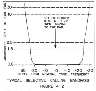
NOTE: The selective calling section is set to trigger with a  $1.5\mu V$  input signal (to attenuator pad) which is within  $\pm 25 Hz$  of the selective calling nominal frequency.
