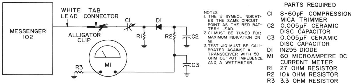
TEST JIG FOR MEASURING
