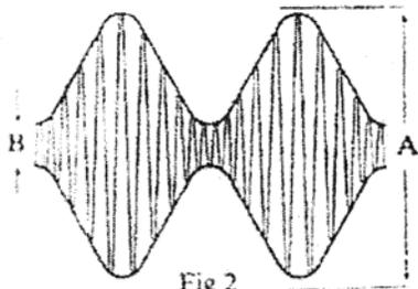
$$\text{Modulation ratio} = \frac{A - B}{A + B} \times 100 [\%]$$
