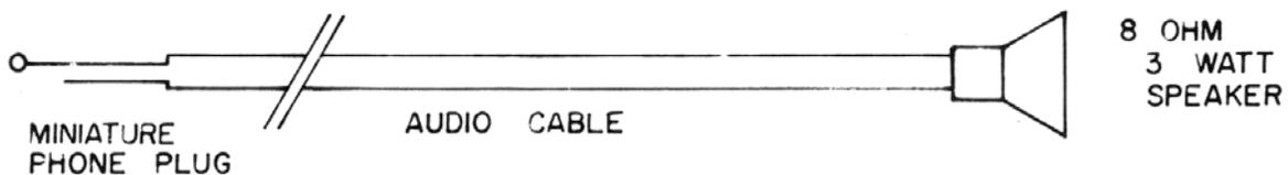
FIGURE 3, P.A. SPEAKER CABLE DIAGRAM
