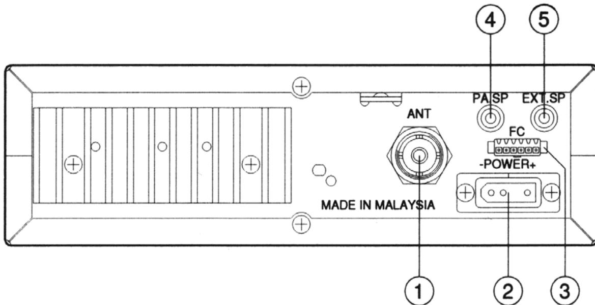
1. **ANTENNA:** This jack accepts a 50 ohm coaxial cable with a PL-259 type plug.
