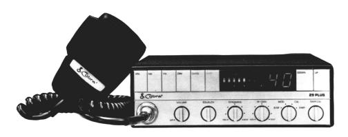
DELUXE MOBILE CB RADIO with ELECTRONIC TUNING 7-SEGMENT BAR GRAPH MULTI-FUNCTION METER "DYNA-MIKE" and CHANNEL SAVER PUSHBUTTON DIRECT/INSTANT TUNING of CHANNELS 9 and 19
