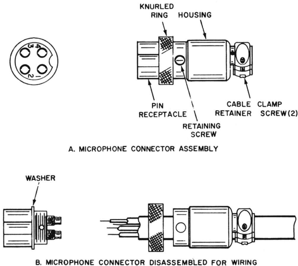
**Fig. 2. Microphone plug wiring**
