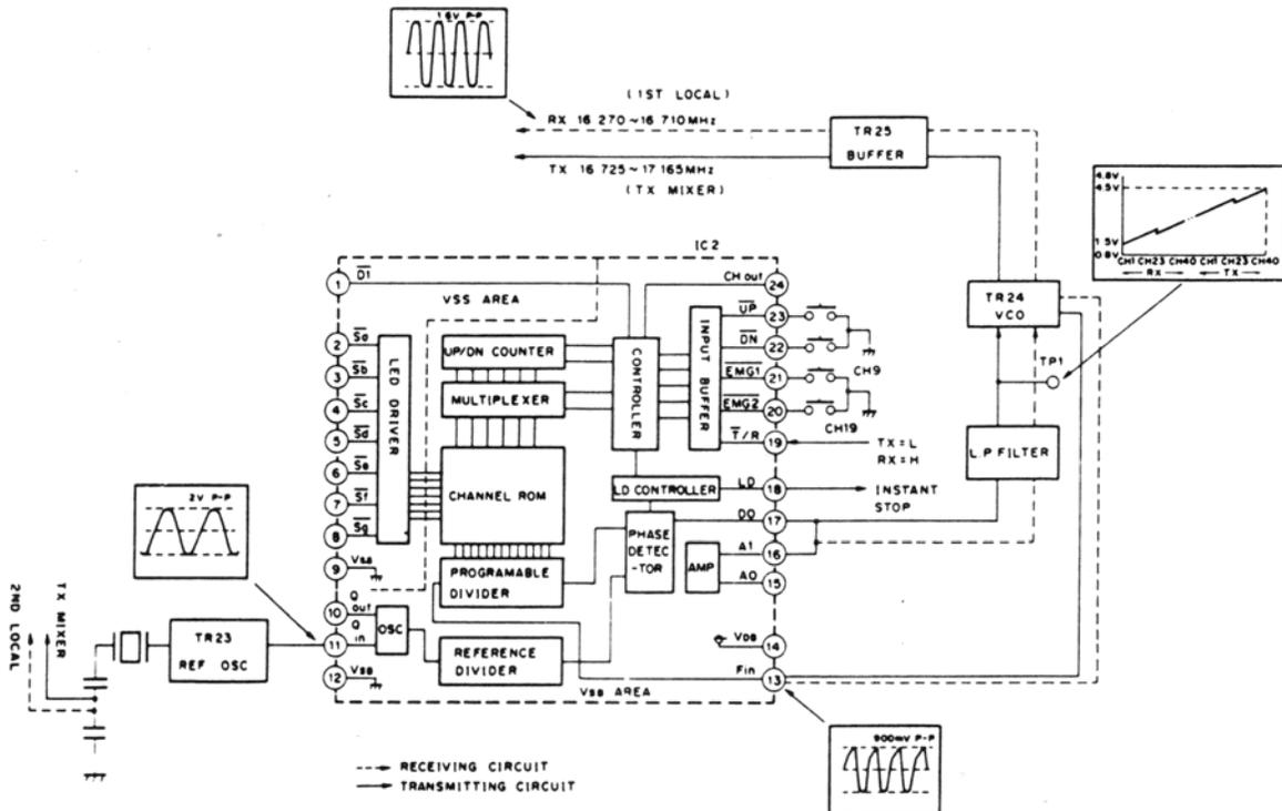
The VCO is an oscillator which controls oscillation frequency in accordance with input voltage change. The VCO output is mixed with a signal in the transmitter or receiver circuitry. A portion of the VCO frequency is fed to IC2 (1/N divider).
