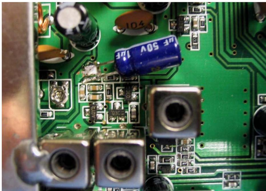
Solder the capacitor as shown. Be sure to observe polarity.
