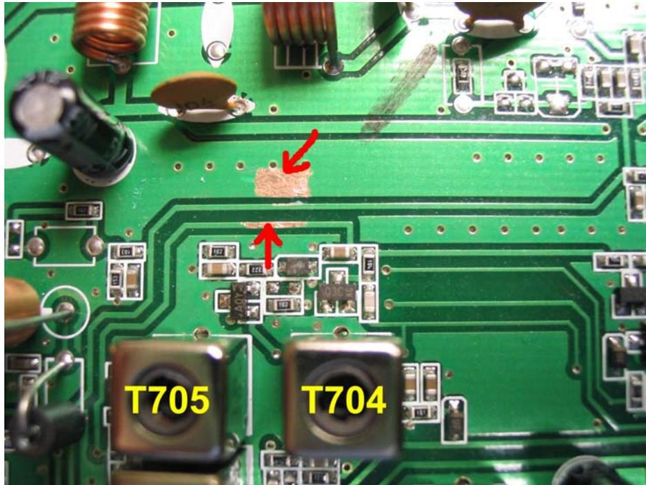
Scrape to expose the circuit traces as indicated above. The large copper area is ground.
