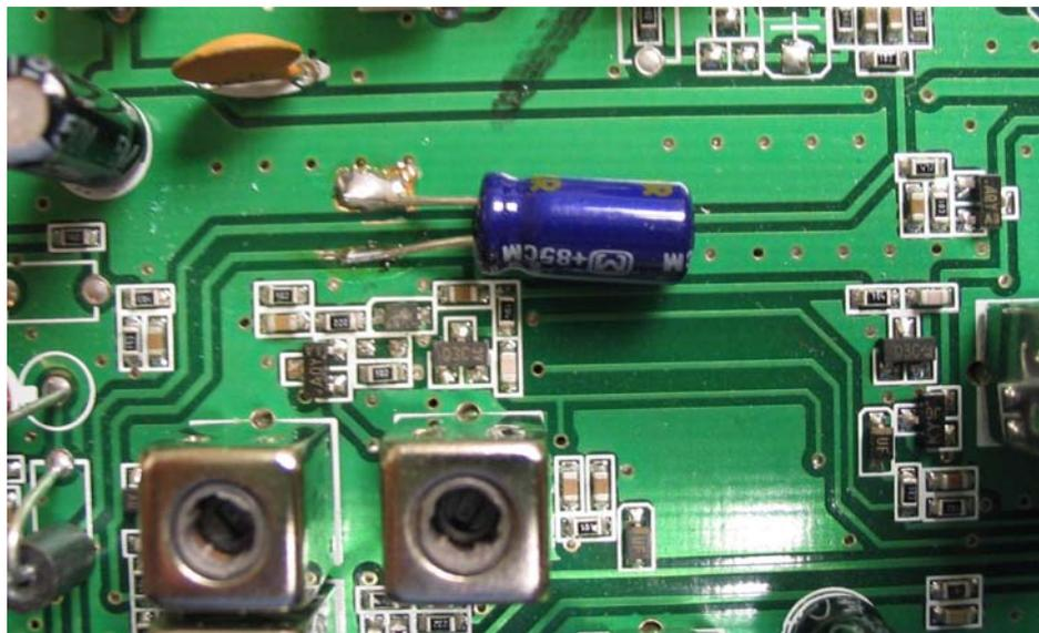
Solder the capacitor as shown. Be sure to observe polarity. Put some glue under the capacitor so that it cannot move.
