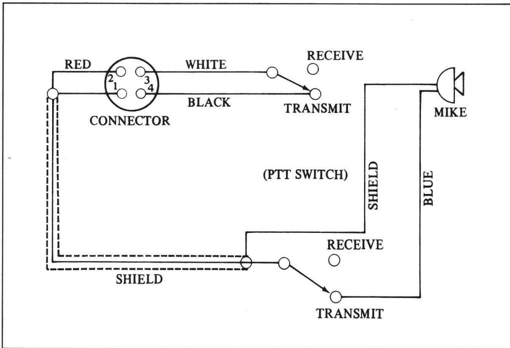
Fig. 3. Microphone and connector wiring diagram.
