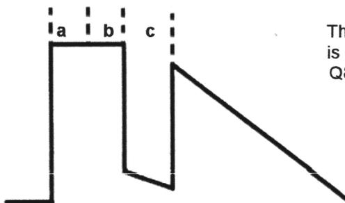
This pulse indicates that the segments for Digit 1 is Open or the cathode is not being grounded by Q801
