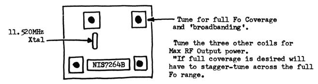
Final results on initial unit: 4W-26.055; 5W-26.315; 6W-26.685; 6.5W-26.955; 6W-27.205; 5W-27.405....
