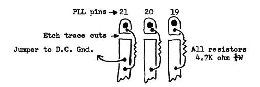
8. Wire dimmer control and ANL switch as shown below: Viewed looking down on trace side of PCB.
